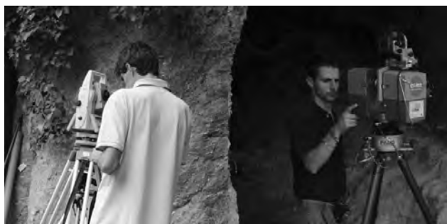
Figure 1. Survey with total station for the cartographic setting of the Re Tiberio cave (left), and laser scanning test with FARO LS PHOTON 20-120 model (right). The survey was carried out with laser scanner Leica HDS6100 (Table 1).
